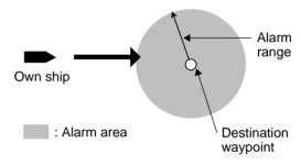
Figure 8-3 How the arrival alarm works
